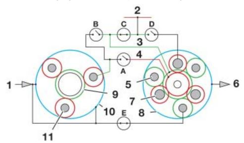
**Power Flow in Reverse Gear:** The drive clutch B is closed in reverse gear. As a result, the sun gear 2 (3) in the double planetary gear train is driven while being in mesh with the long planet gears. The double planet carrier is supported by brake clutch D and the gear-box housing. The internal gear 2 (output shaft) can now be driven by the long planet gears in the *opposite direction* of engine rotation (large gear reduction).
